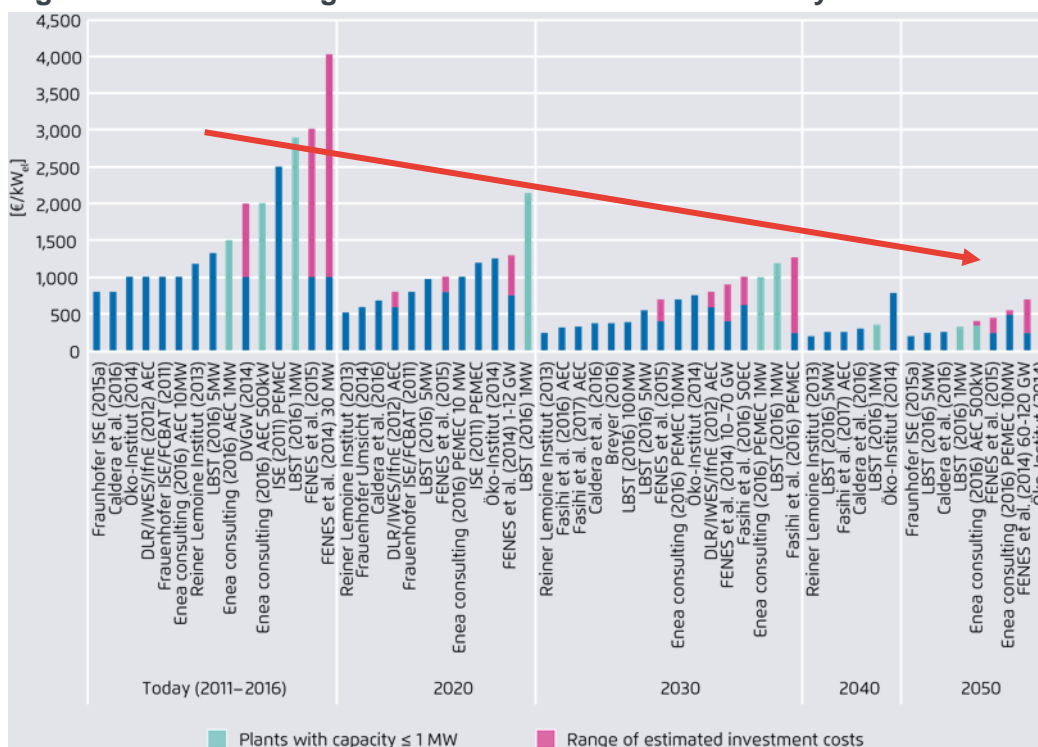
Figure 28 Decreasing investment cost for water electrolysis until 2050
